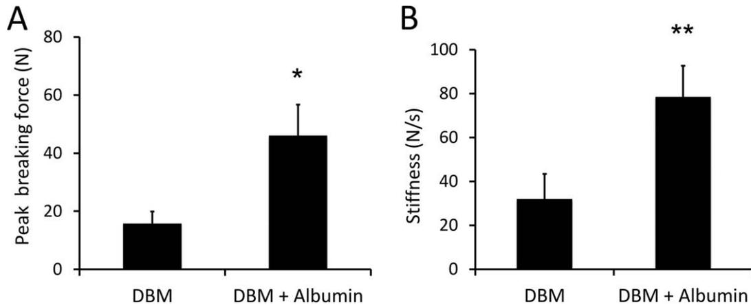
**FIGURE 5.** *Ex vivo* mechanical push-out testing at 11 weeks. Panel A shows peak breaking force (N) of the implanted material. Panel B shows the stiffness (N/mm<sup>2</sup>) of the implanted material. Significantly higher breaking force and stiffness can be seen in the albumin coated group (Unpaired t test, \*:  $p < 0.05$ ).
